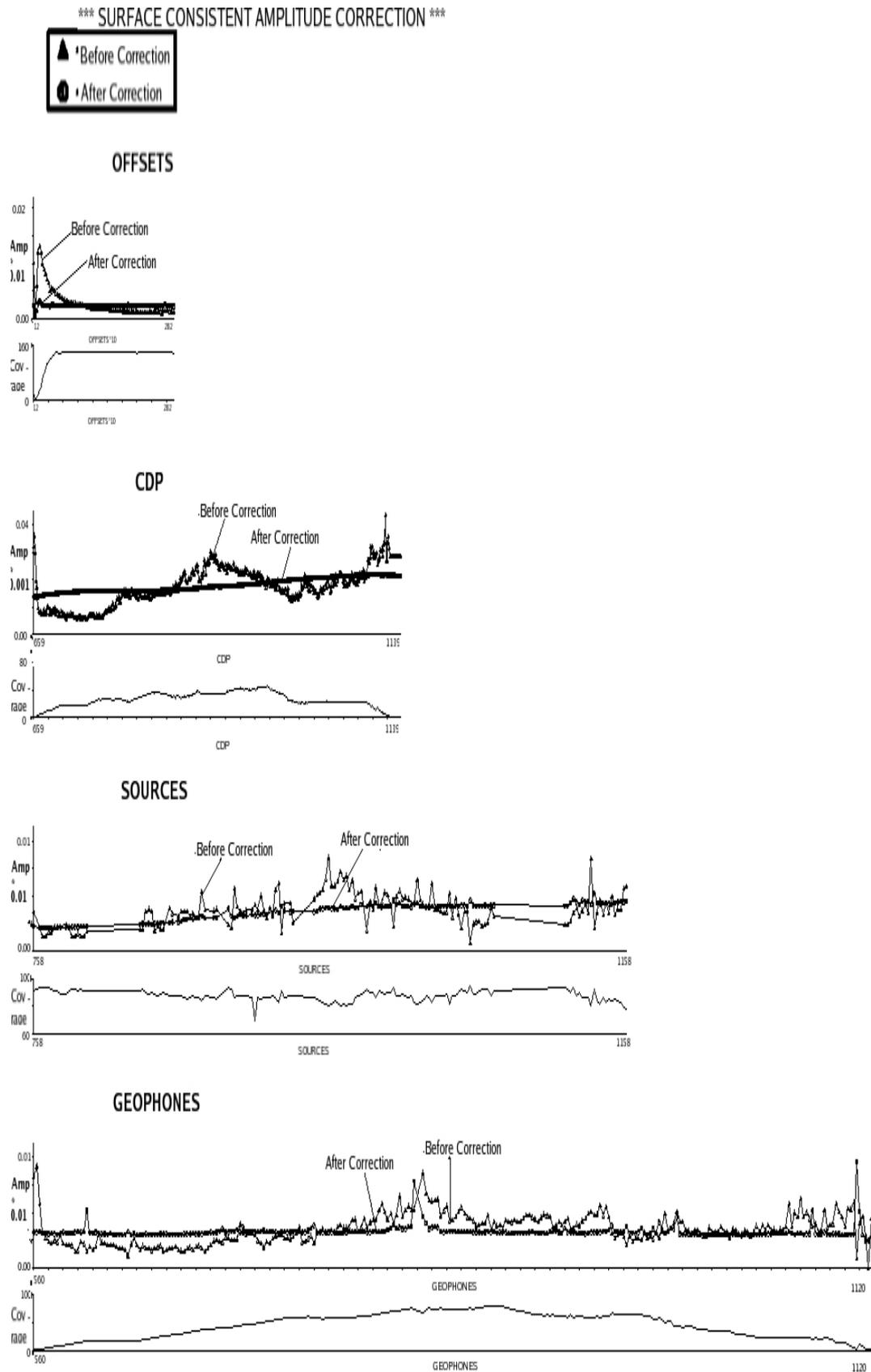
Figure 1. Surface Consistent Correction on data set for different components without time gain application i.e. Stream-2
